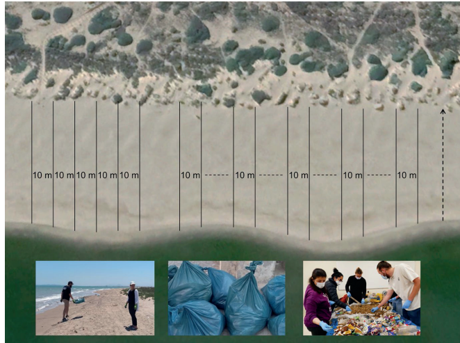
Fig. 2 Macro-litter surveys on the beach. On the left side, the 10 m transects were positioned directly next to each other (Tunisia and Egypt). On the right side, larger space of 10–150 m (horizontal dashed line) was used between transects, depending on the length of the beach (Morocco). Vertical dotted black line (on the far right) indicates the Sand Rake method used in direct proximity. The bottom pictures show the survey procedure, which includes systematic litter collection on the beach, placing the litter in plastic bags, and subsequently counting and categorizing the collected litter in the laboratory
