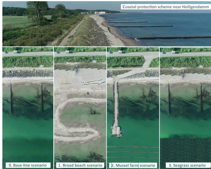
Figure 3. Simplified visualization of the building-with-nature scenarios in front of the Converter lowland near Heiligendamm used in the ecosystem service assessment: the present situation as (0) baseline scenario, (1) scenario with an extended nourished beach, (2) scenario with pier and mussel farm and (3) scenario with seagrass ( Zostera spp. ) and submerged macrophytes in front of the beach.
